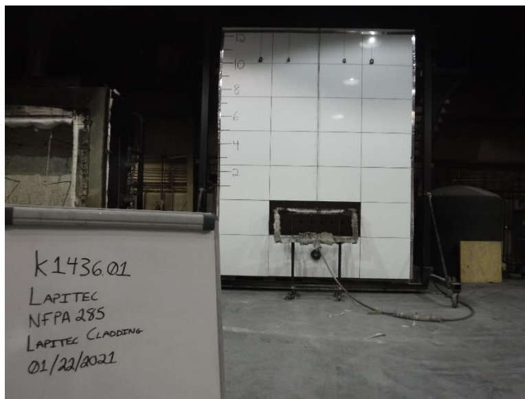
Photo No. 14 Completed Assembly (Pre-test)
