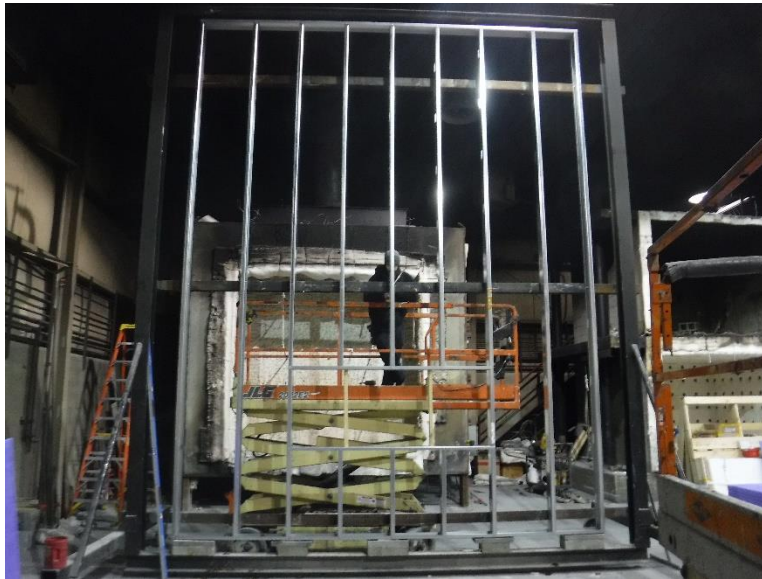
Photo No. 1 Core Wall Framing Completed
