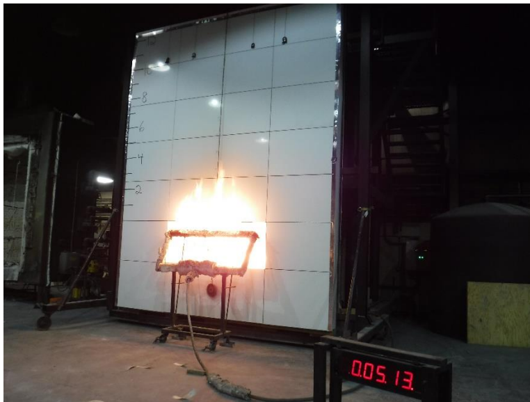
Photo No. 16 Ignition of Window Burner
