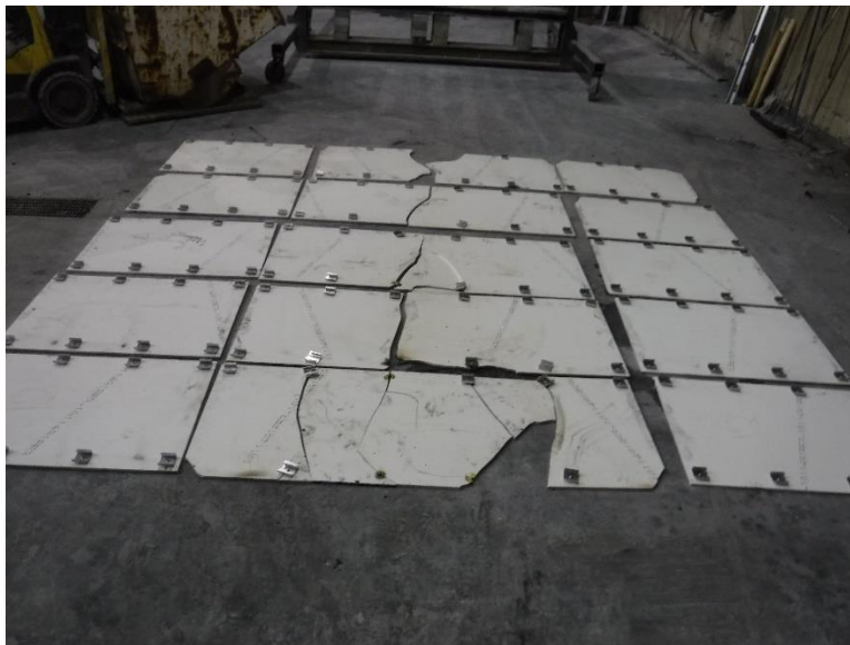
Photo No. 22 Unexposed Side of Exterior Cladding
