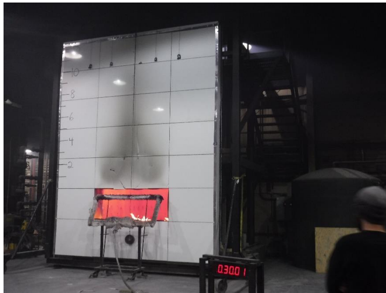
Photo No. 17 Burners Extinguished
