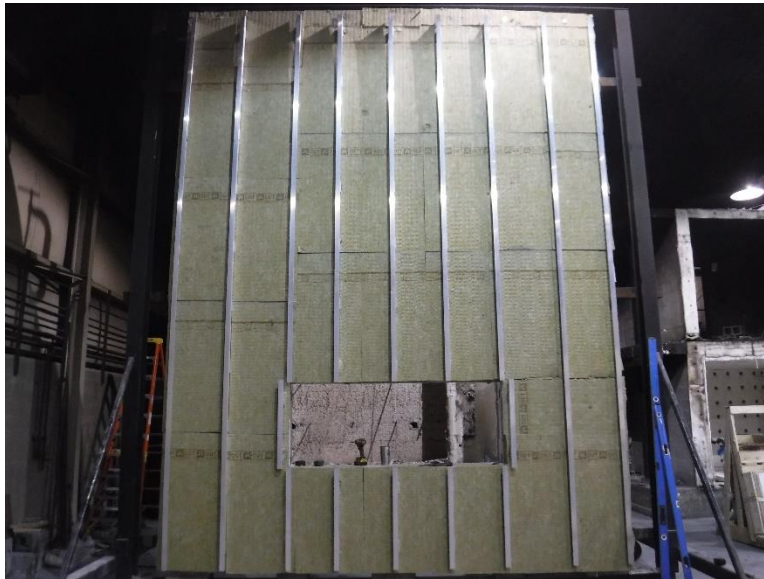
Photo No. 7 L-Profiles Installed
