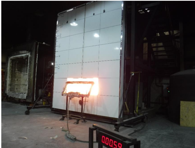
Photo No. 15 Ignition of Room Burner
